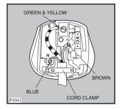
The wire coloured green and yellow must be connected to the terminal marked with the letter  $\times E$  or by the earth symbol  $\frac{1}{=}$  or coloured green and yellow.
